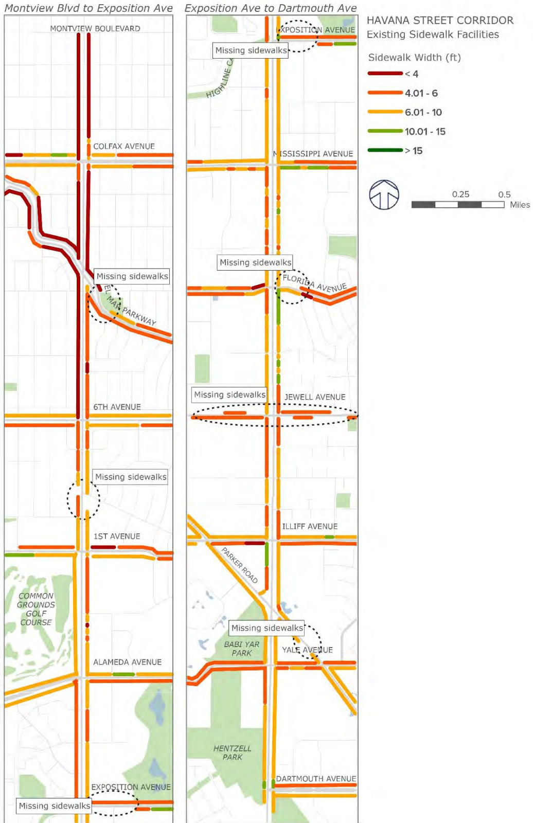
Figure 3.4.2: Existing Sidewalk Facilities
